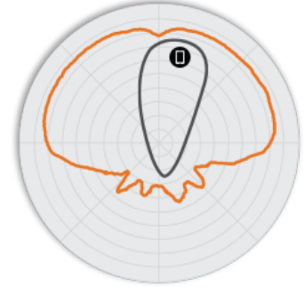
Figure 5. H320 5GHz Elevation Antenna Patterns
