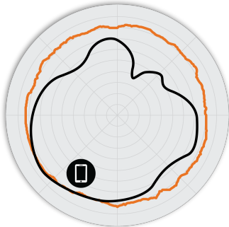
Figure 2. M510 2.4GHz Azimuth Antenna Patterns
