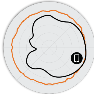
Figure 3. M510 5GHz Azimuth Antenna Patterns
