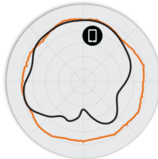
Figure 3. R320 5GHz Azimuth Antenna Patterns
