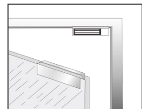
13 Screw door After all the appropriate procedures, the holding force can be maximized. Finally, fix the tamper screw.
