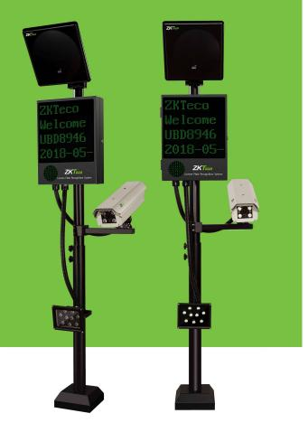
LPRS2000 is a hybrid identification vehicle management terminal that adopts multiple recognition modes for long-range RFID and license plate recognition. And compare to the traditional license plate recognition product, it combines the latest developed high-performance UHF reader to ensure that the capture rate and recognition accuracy of fixed vehicles are up to 100%.
